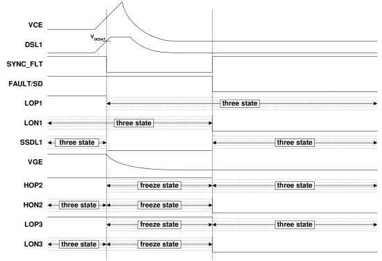
Figure 6: Example of a desaturation detection event
