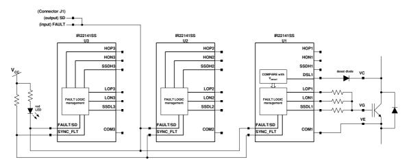
Figure 5: Three phase connection
