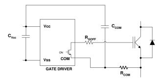
Figure 10: COM below ground protection
