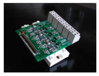
IR2214SS Demo Board (Shown with optional IGBT Power Module)
