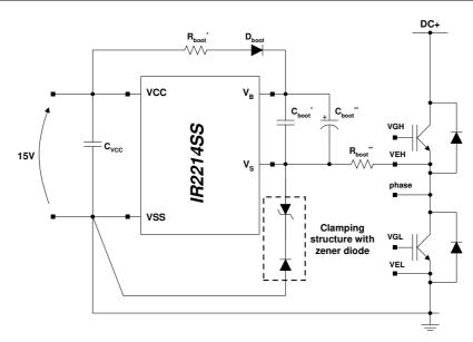
Figure 9: -V<sub>s</sub> clamp
