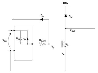
Figure 11: Collector-Gate current protection
