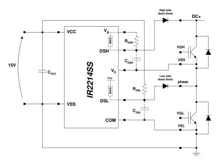
Figure 8: Desat external filter
