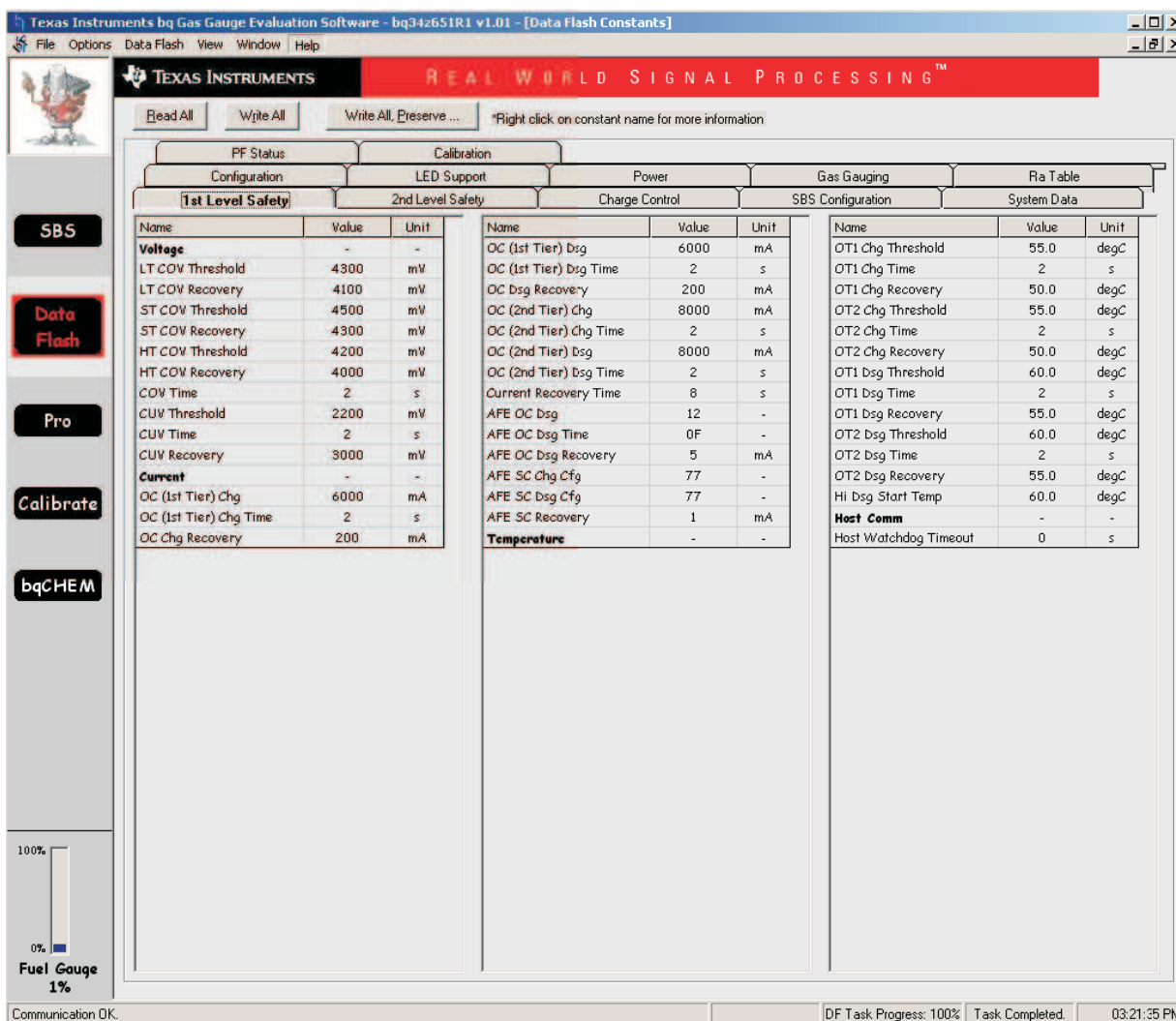
Figure 9. Data Flash Screen, 1st Level Safety Class
