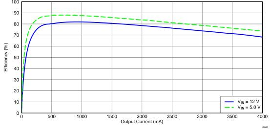
Figure 1 shows the efficiency for the TPS54427 at an ambient temperature of 25°C.
