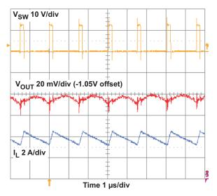
Figure 6. TPS54427 Output Voltage Ripple
