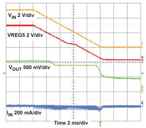
Figure 9. TPS54427 Shut-down Relative to V<sub>IN</sub>
