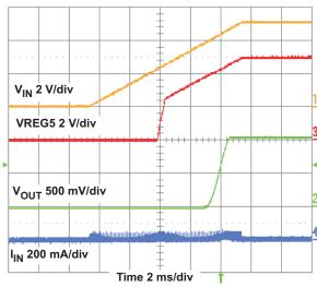
Figure 8. TPS54427 Start-Up Relative to V<sub>IN</sub>
