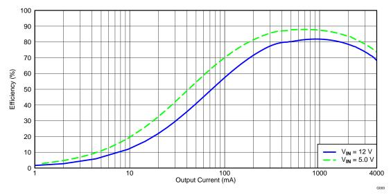
Figure 2. TPS54427 Light-Load Efficiency
