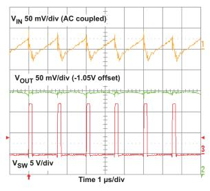
Figure 7. TPS54427 Input Voltage Ripple
