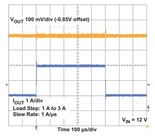
Figure 5. TPS54427 Load Transient Response
