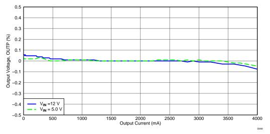
Figure 3. TPS54427 Load Regulation,  $V_{IN} = 5$  V and  $V_{IN} = 12$  V.
