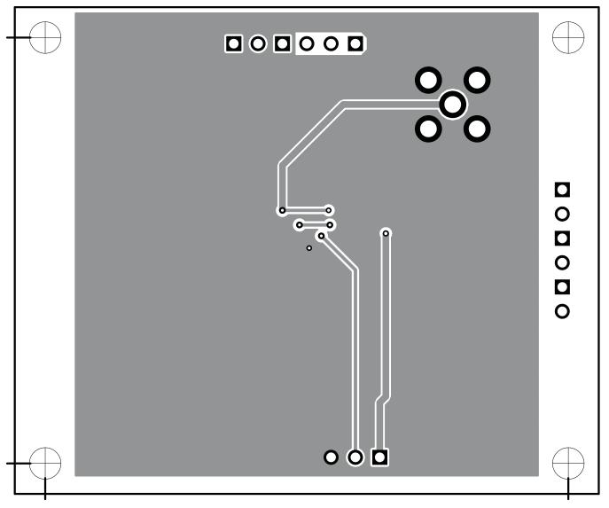
Figure 13. TPS62122EVM Bottom-Side Copper (Bottom View)
