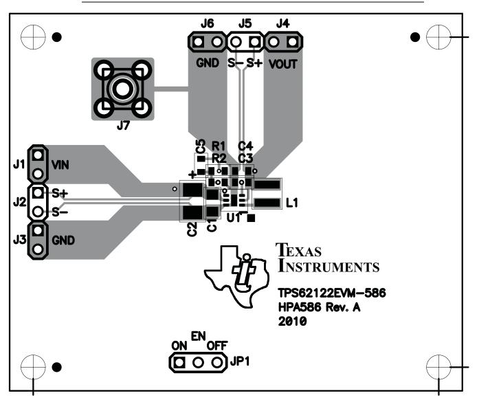
Figure 11. TPS62122EVM Component Placement (Top View)
