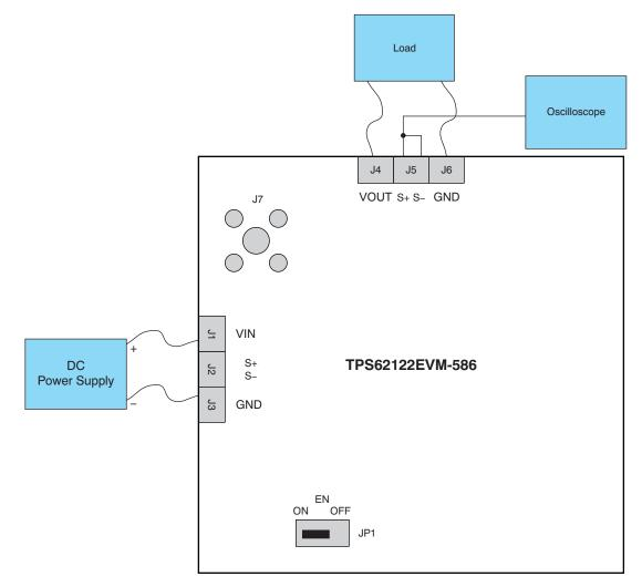
Figure 2. Hardware Board Connection
