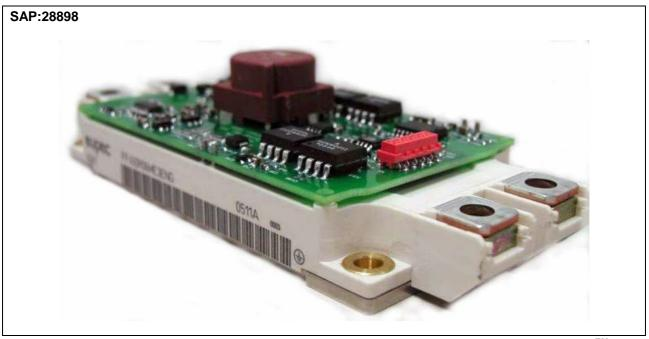
Figure 1 The 2ED100E12-F Evaluation Driver Board mounted on the top of the EconoDUAL<sup>™</sup> module
