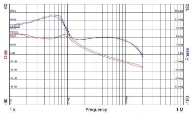
*Figure 2- Satisfactory frequency response of typical application circuit shown on page 1.* Crossover frequency fc is about 35kHz with a corresponding phase margin of 60 degrees. The two sets of curves, which are essentially identical, correspond to load current of 1A and 2.5A.
