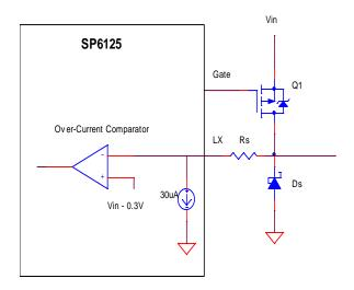
Figure 3- Overcurrent protection circuit
