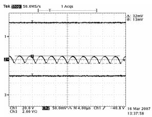
Figure 10- Output ripple at 3A is 32mV, ch1: VIN; ch2: VOUT; ch3: IOUT
