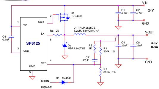
Figure 4- Application circuit for Vin=24V
