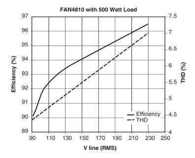
Figure 1. FAN4810 Evaluation Board Test Results
