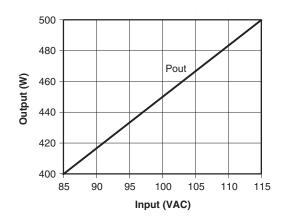
Figure 2. Output Power vs. Line Voltage
