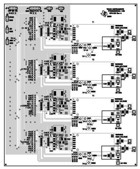
Figure 7. Assembly Layer
