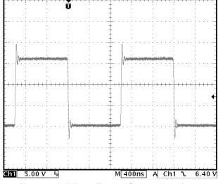
Figure 6 - IXDD404 Typical Output Waveform F=500KHz, CL=1800pF
