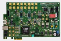
The LatticeECP3 Serial Protocol Board provides a platform to evaluate the LatticeECP3 device's multi-protocol serial protocol functionality as well as DDR2 and DDR3 memory interfaces.
