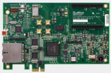
The LatticeECP3 Versa Evaluation Board is the industry's lowest cost FPGA board with PCI Express and two Gigabit Ethernet ports. It is useful for appreciating the quality of LatticeECP3 SERDES and developing a wide-range of networking and system design applications.
