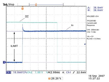
Figure 10. TPS2051BEVM-290 Short-Circuit Output Current and OC Status
