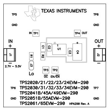
Figure 3. TPS20xxEVM-290 Component Placement
