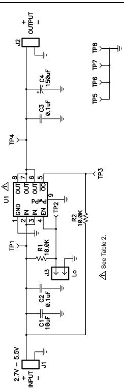
Figure 2. TPS20xxEVM-292 Schematic
