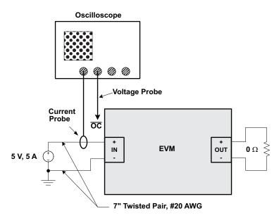
Figure 9. EVM Setup For Measuring Current Limit
