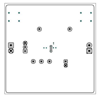
Figure 5. Bottom Copper (top view)
