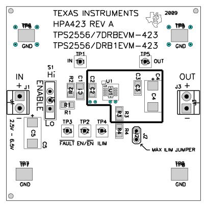
Figure 3. Top Layer Assembly (top view)
