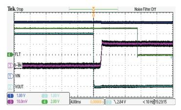
Figure 2. 100-kΩ R<sub>ILIM</sub> Enabled Into a Short Circuit
