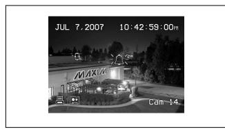
Figure 1. CVBSOUT with the First OSD Display in Demo Mode (NTSC)
