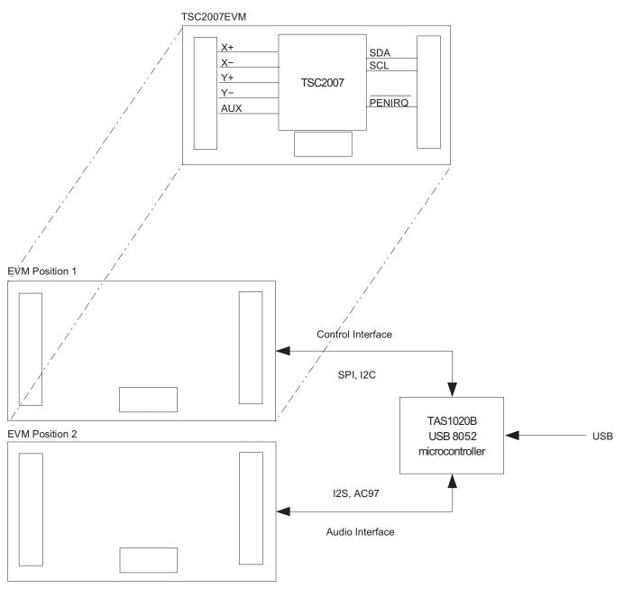
Figure 1. TSC2007EVM-PDK Block Diagram
