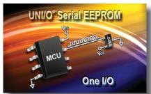
Microchip's new UNI/O serial EEPROM family uses only ONE connection to the host microcontroller. This compares to two or three pins for I<sup>2</sup>C. and three to six
