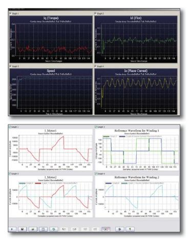
Real-Time Data Monitor (RTDM) – Make a change to a software parameter and see the effect immediately without stopping the motor. A serial USB or UART cable supports bi-directional data transfers between the host PC and the MCU/DSC. This is configured within DMCI and most motor control application note software comes with a setup file to automatically configure RTDM for the application.
