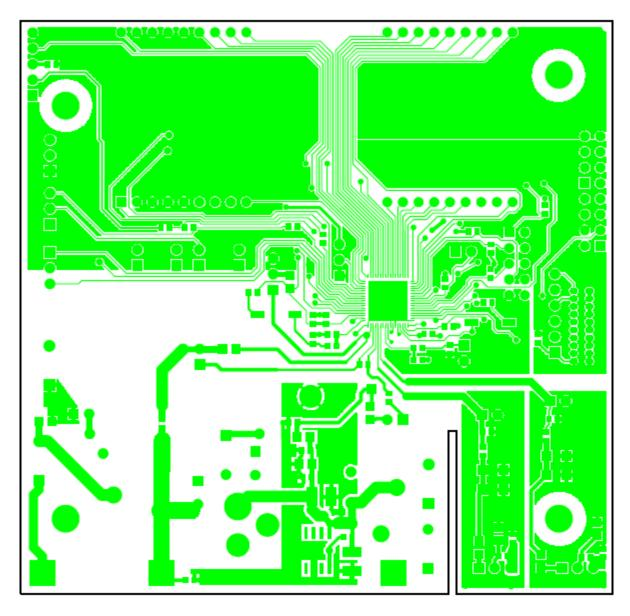
Figure 4-5: 71M6531N12A2 Demo Board: Top Copper Layer
