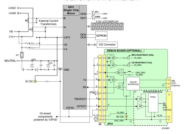
Figure 1-3: The TERIDIAN 6531 Demo Board with Debug Board Block Diagram (CT Configuration)
