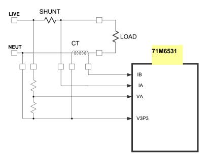
Figure 2-7: 71M6531 with Shunt and CT
