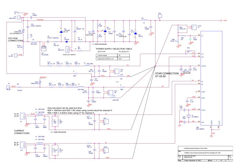
Figure 4-1: 71M6531N12A2 Demo Board (REV 2.0): Electrical Schematic 1/3 – Shunt Configuration
