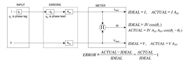
Figure 2-1: Watt Meter with Gain and Phase Errors.
