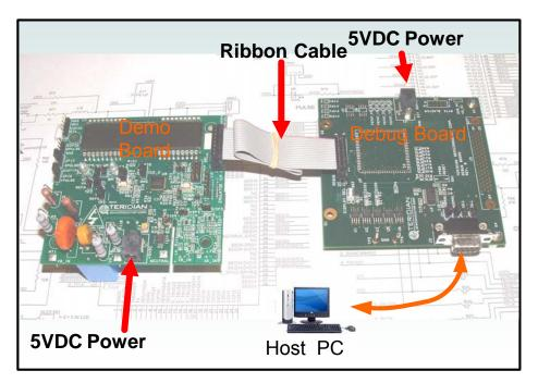
Figure 1-2: Demo Board: Ribbon Cable Connections
