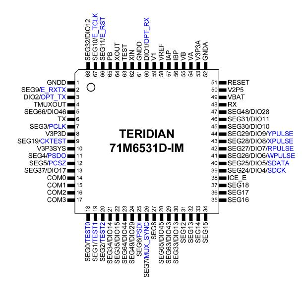
Figure 4-16: TERIDIAN 71M6531D/F LQFP64: Pinout (top view)
