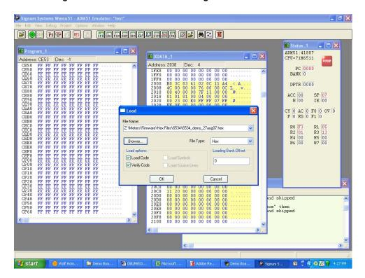
Figure 1-10: Emulator Window Showing Erased Flash Memory and File Load Menu
