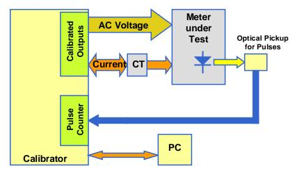
Figure 2-8: Meter with Calibration System
