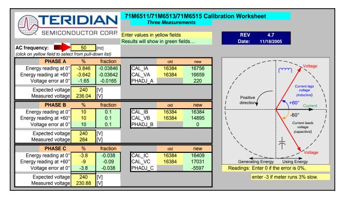
Figure 2-3: Calibration Spreadsheet for Three Measurements
