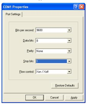
Figure 1-4: Port Configuration Setup
