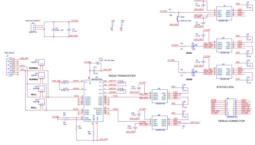
Figure 4-9: Debug Board: Electrical Schematic
