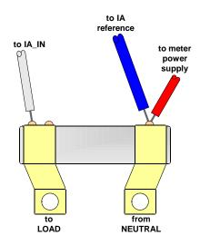
Figure 1-6: Pre-wired shunt resistor
