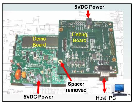
Figure 1-1: Demo Board: Basic Connections
