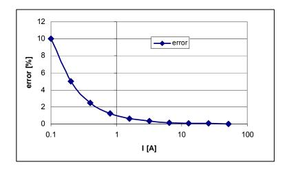
Figure 2-6: Non-Linearity Caused by Quantification Noise
