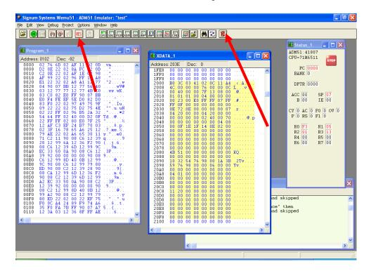
Figure 1-9: Emulator Window Showing Reset and Erase Buttons
