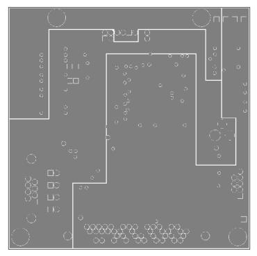
Figure 4-13: Debug Board: Middle Layer 1, Ground Plane
