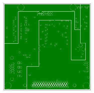
Figure 4-14: Debug Board: Middle Layer 2, Supply Plane
