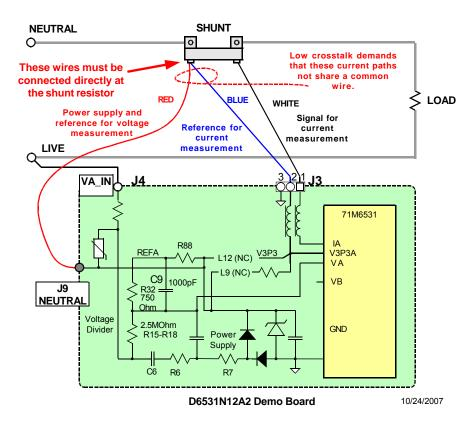
Figure 1-7: Connection of the Pre-Wired Shunt Resistor
