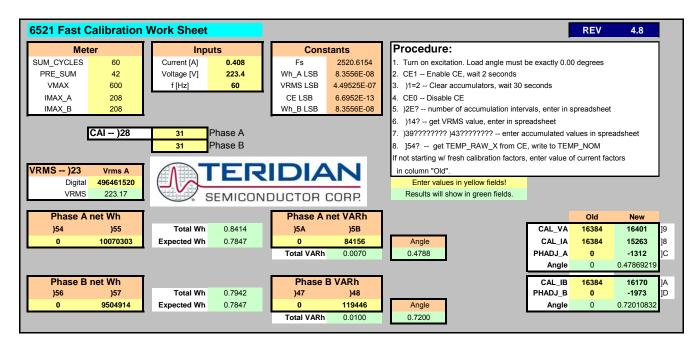
Figure 2-5: Calibration Spreadsheet for Fast Calibration
