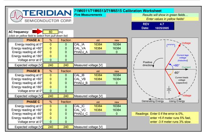
Figure 2-4: Calibration Spreadsheet for Five Measurements
