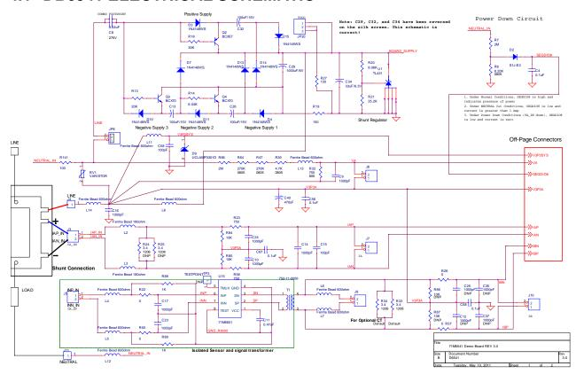
Figure 4-1: DB6541 REV 3.0 Demo Board: Electrical Schematic ½
