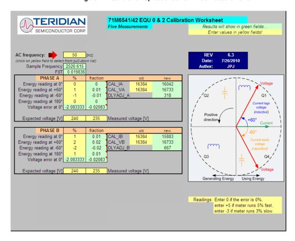
Figure 2-8: Calibration Spreadsheet for Five Measurements
