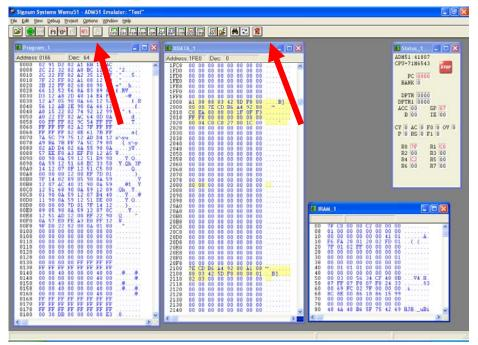
Figure 1-5: Emulator Window Showing Reset and Erase Buttons (see Arrows)
