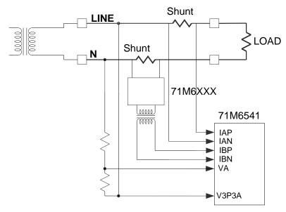
Figure 2-3: Single-Phase Two-Wire Meter with two Shunt Sensors
