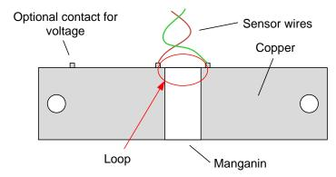
Figure 2-17: Loop Formed by Shunt and Sensor Wire
