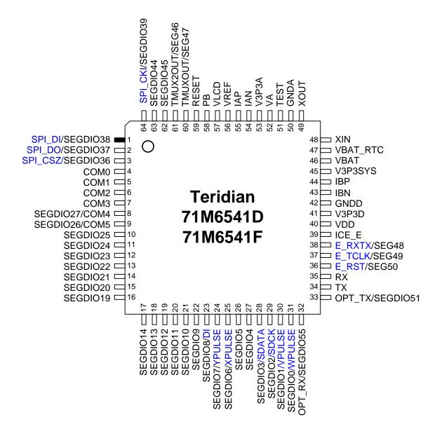
Figure 4-7: Teridian 71M6541F, LQFP64: Pin-out (top view)
