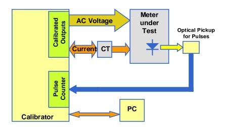
Figure 2-12: Meter with Calibration System
