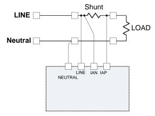
Figure 2-1: Shunt Connections
