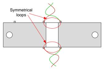
Figure 2-18: Shunt with Compensation Loop
