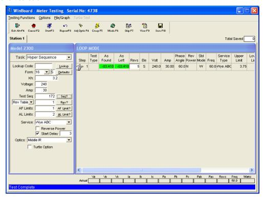
Figure 2-13: Calibration System Screen
