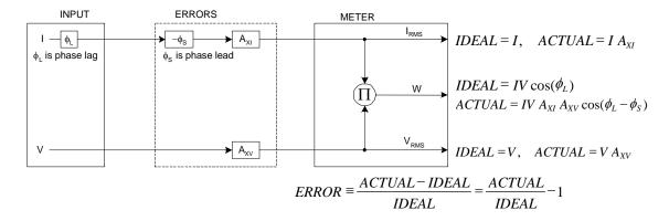
Figure 2-5: Watt Meter with Gain and Phase Errors.
