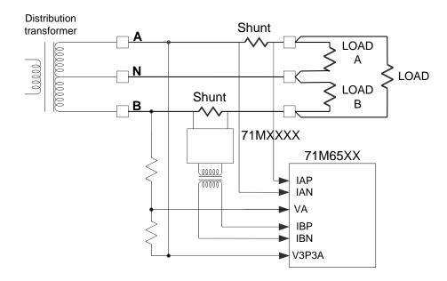
Figure 2-4: Single-Phase Three-Wire Meter with two Shunt Sensors
