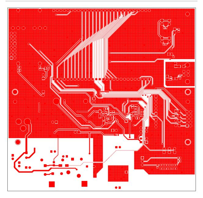
Figure 4-6: DB6541 REV 3.0: Bottom Copper
