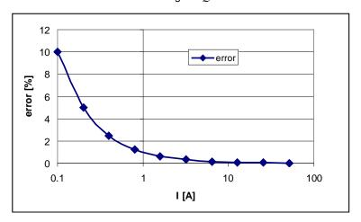
Figure 2-9: Non-Linearity Caused by Quantification Noise
