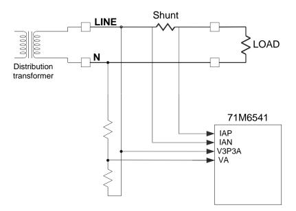
Figure 2-2: Single-Phase Two-Wire Meter with Shunt Sensor
