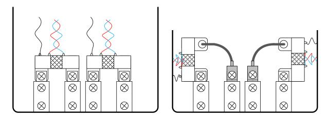
Figure 2-15: Typical Sensor Arrangement (left), Recommended Arrangement (right)
