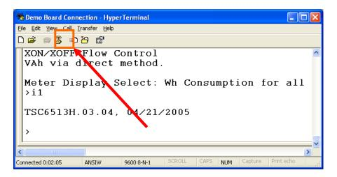
Figure 1-2: HyperTerminal Sample Window with Disconnect Button (Arrow)
