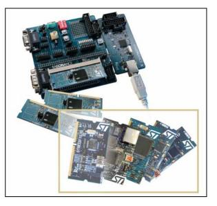
evaluation board, microcontrollers, embedded RLink JTAG in-circuit debugger/programmer and Raisonance Integrated Development Environment (RIDE).
