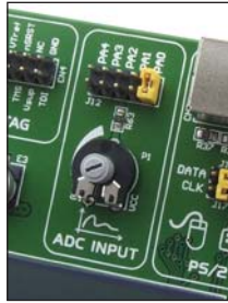
Figure 11-2: The PA0 pin used as A/D conversion input
