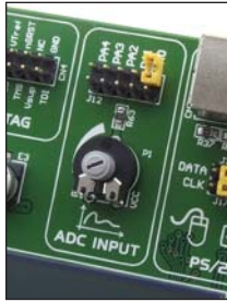
Figure 11-1: ADC (default jumper positions)
