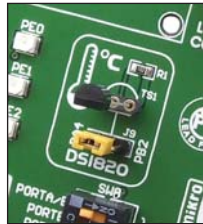
Figure 10-2: J9 in the left-hand position (1-wire communication through the PA4 pin)
