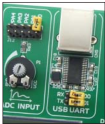
Figure 9-1: USB UART module (J16 and J17 are not placed)
