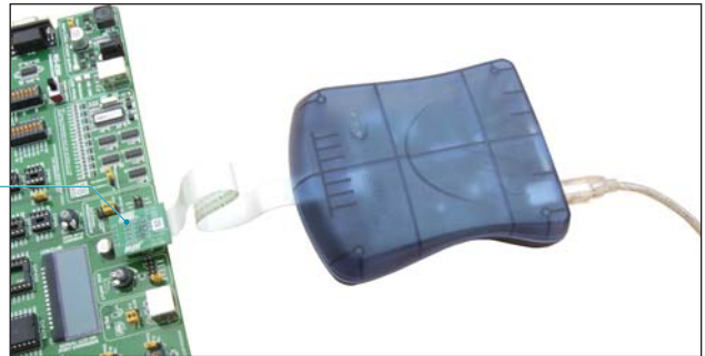
Figure 5-2: JTAGICE mkII connected to the development system
