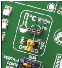
Figure 10-1: DS1820 in the connector (1-wire communication is not used)
