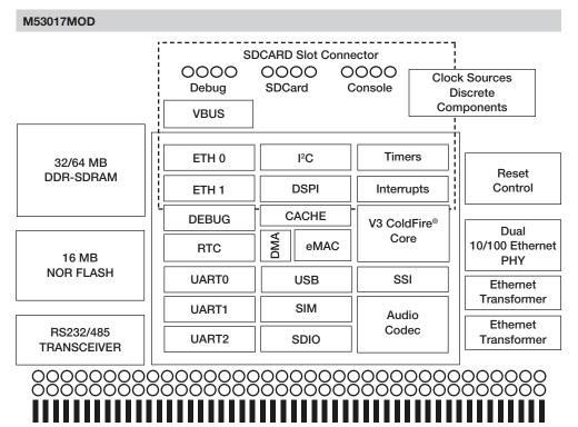
60 PIN EDGE CONNECTOR OR HEADER BUS
