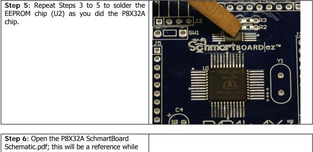
Schematic.pdf; this will be a reference while assembling. Each of the parts that you will install from here out will need the appropriate portions of solder and flux; depending on the type of solder you use will determine the heat needed for the soldering iron; please see solder package for details. The SchmartBoard uses lead-free solder and is suggested as the type to use.
