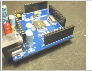
**Step 12**: Carefully clean off any extra flux that may be on the board and allow to fully dry before connecting to power or programming tool.
