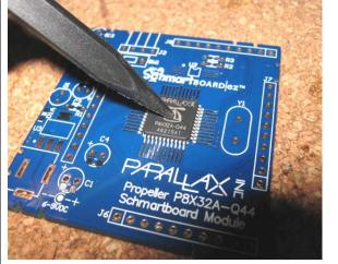
**Step 4**: Carefully solder each chip leg to the SchmartBoard, by pushing the solder from the outside of the groove to the chip leg; hold iron by pad about 2-3 seconds.
