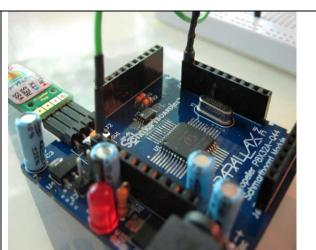
Step 16: Run this test code that blinks the LED on I/O pin P23 to confirm operation. Change the Pin constant and circuit to test the rest of the I/O pins.
