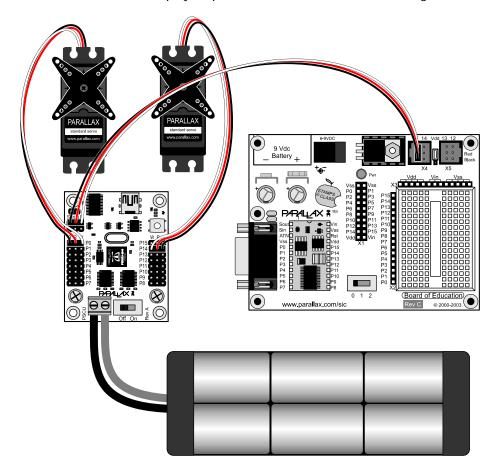
The PSCU is shown here connected to a Board of Education, two servos, one connected to channel 0 and the other connected to channel 14 and a 7.2 V R/C battery back. The 7.2 V R/C battery pack provides power for the servos.
