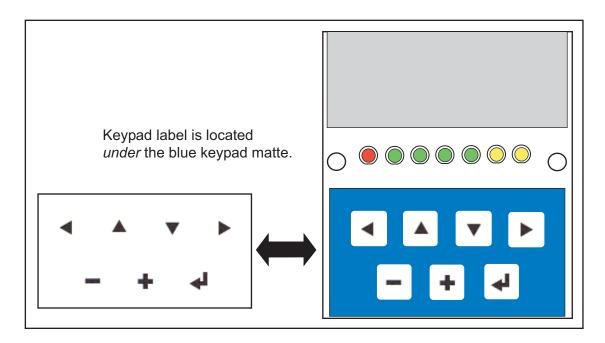
Figure D-5. Removing and Inserting Keypad Label
