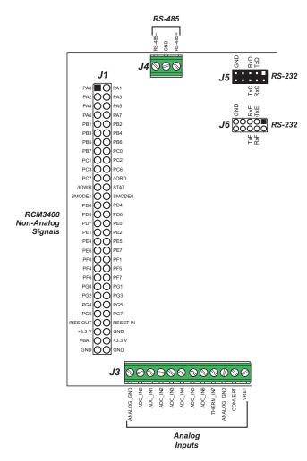
Figure B-4. Prototyping Board Pinout
