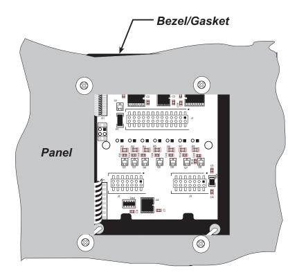
Figure D-9. LCD/Keypad Module Mounted in Panel (rear view)
