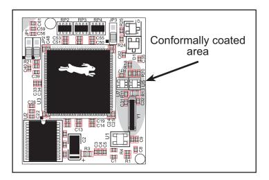
Figure A-5. RCM3400 Areas Receiving Conformal Coating
