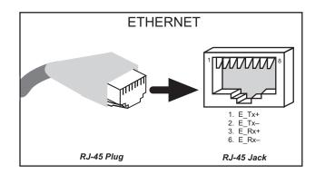
Figure B-10. RJ-45 Ethernet Port Pinout
