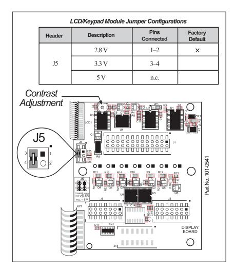
Figure D-3. LCD/Keypad Module Voltage Settings
