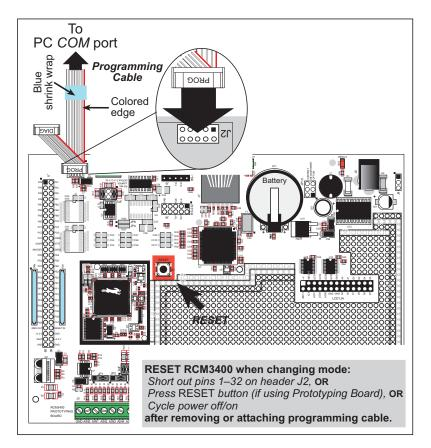
Figure 7. Switching Between Program Mode and Run Mode
