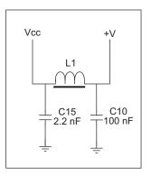
Figure 11. Analog Supply Circuit
