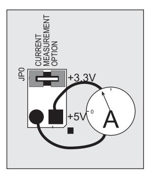
Figure B-5. Prototyping Board Current-Measurement Option
