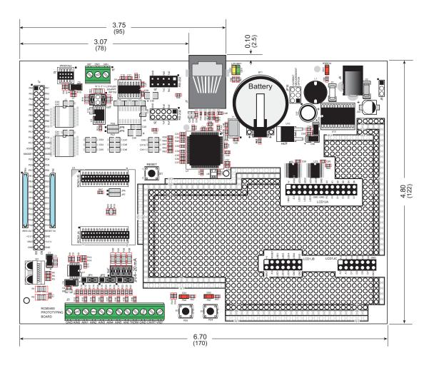
Figure B-2. Prototyping Board Dimensions
