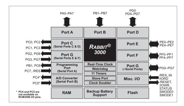
Figure 6 shows the use of the Rabbit 3000 microprocessor ports in the RCM3400 modules.
