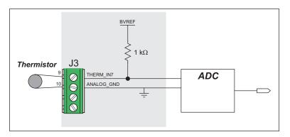
Figure B-7. Prototyping Board Thermistor Input
