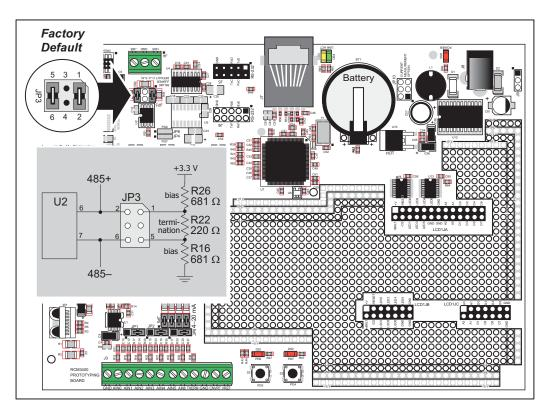
Figure B-9. RS-485 Termination and Bias Resistors
