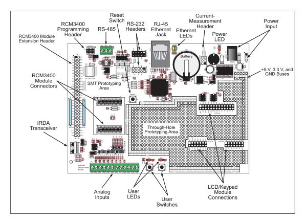
The Prototyping Board is shown below in Figure B-1, with its main features identified.
