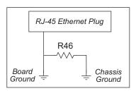
Figure B-11. Isolation Resistor R46
