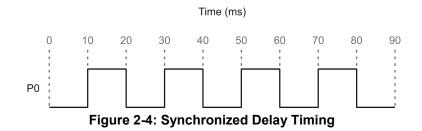
Using the synchronized delay method, our output signal is always perfectly aligned to the time base plus a multiple of our interval. This will work as long as the time base (an external crystal) is accurate and the overhead in the loop does not exceed the time interval itself. Note that we waited, with WAITCNT, before the first toggle so that the time between the very first toggle and the second matches that of all the rest.
