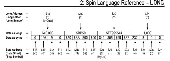
Figure 2-2: Main Memory Long-Sized Data Structure and Addressing
