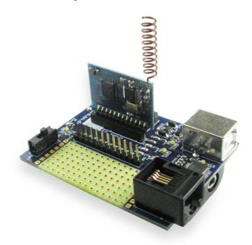
The EZLink Development Kit provides a complete, ready-to-use RF module solution through the industry-leading EZRadio technology. A single-chip, low-power solution, the IA4421 is a 434, 868 and 915 MHz multi-channel, Frequency-Shift Keying (FSK) transceiver that is designed to provide the industry's lowest radio BOM by using only one external component—a crystal. The
