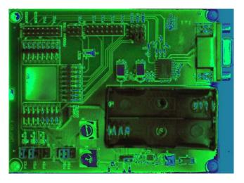
Figure 2-2. Top Side of FreeStar Interface Board
