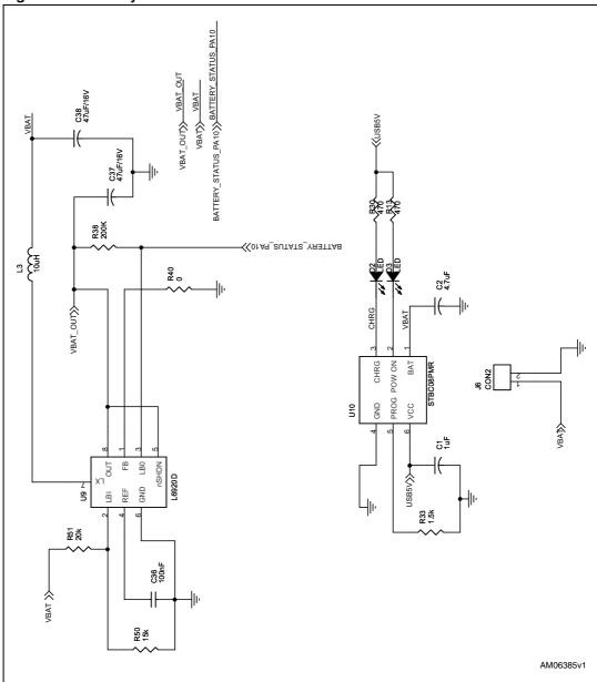
Figure 4. Battery circuit schematics
