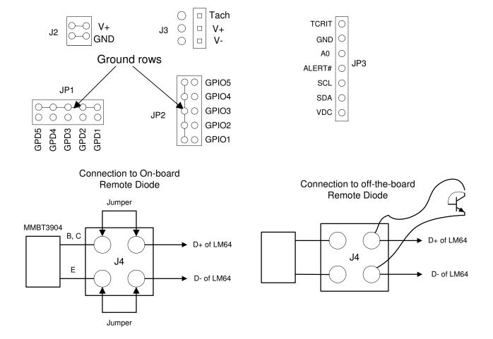
Figure 3. Header Connectors on the LM64 Evaluation Board
