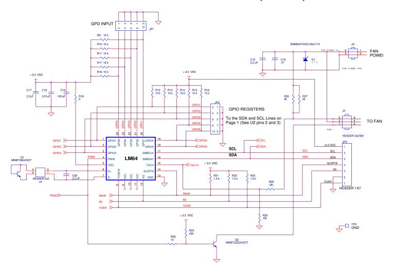
Figure 5b. Schematic of LM64 Evaluation Board - Page 2 of 2
