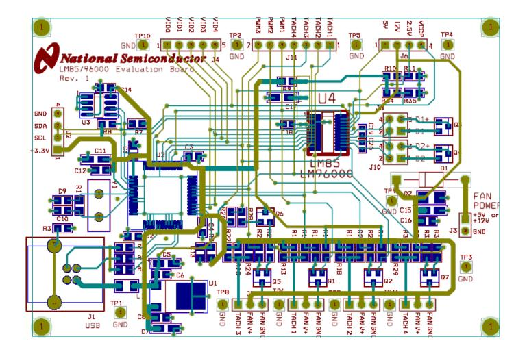
Figure 5.3 Layout diagram of the LM85/LM96000 Evaluation Board
