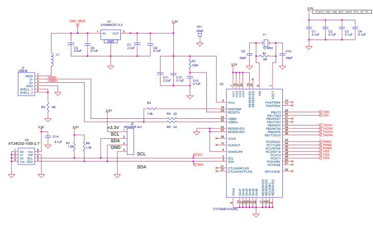
Page 1 of 2 Pages of the Schematic of the LM85/LM96000 Evaluation Board
