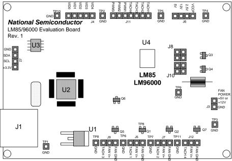
Figure 2.1.1 Physical Layout of the LM85/LM96000 Evaluation Board
