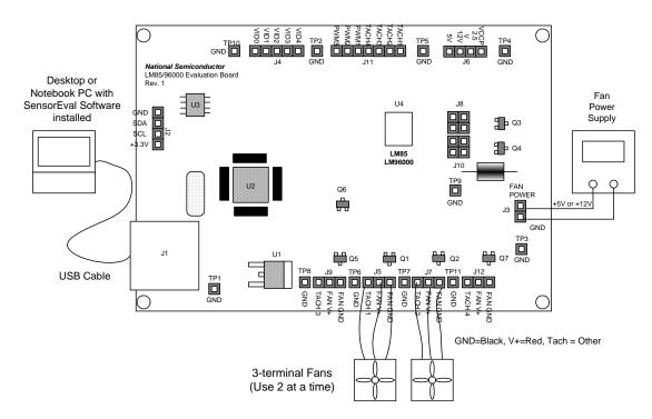
Figure 2.1.2 Wiring Diagram showing Hookup of the LM85/LM96000 Evaluation Board
