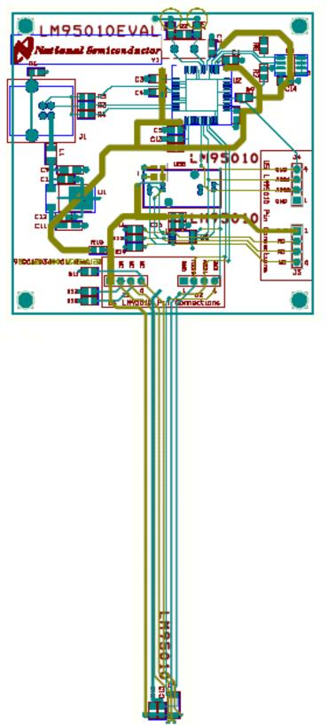
Figure 5.3 Layout diagram of the LM95010 Evaluation Board
