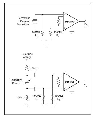
FIGURE 3. Providing An Input Bias Current Path.
