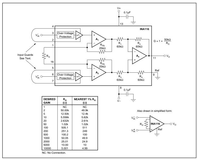
FIGURE 1. Basic Connections.
