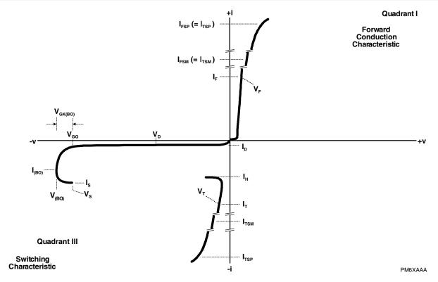
Figure 1. Voltage-Current Characteristic
