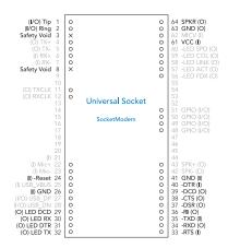
**Universal Socket Connectivity.** Multi-Tech's universal socket flexible comm-port architecture provides analog dialup, ISDN, wireless, or Ethernet socket connectivity with interchangeable communications devices. This allows you to utilize one system design and populate it with your communications device of choice. In addition, you are assured a seamless migration to future technologies.
