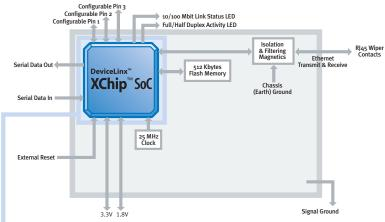
Note: OEM supplies Flash Memory, RJ45-Magnetics, Clock crystal and regulated power inputs.
