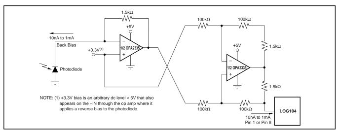
FIGURE 8. Precision Current Inverter/Current Source.
