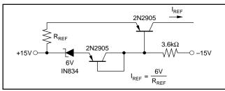
FIGURE 3. Temperature Compensated Current Source.
