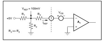
FIGURE 4. T Network for Reference Current.
