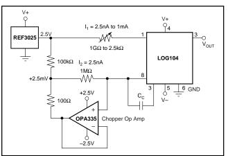
FIGURE 5. Current Source with Offset Compensation.
