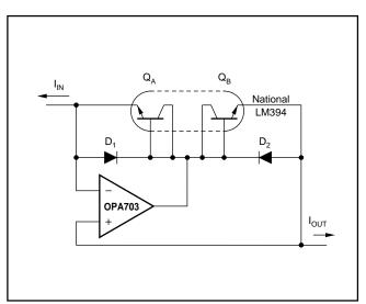
FIGURE 6. Current Inverter/Current Source.
