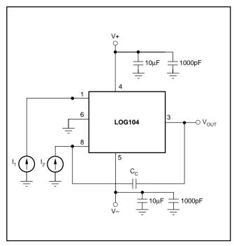
FIGURE 1. Basic Connections of the LOG104.
