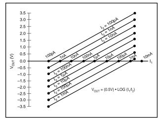
FIGURE 13. Transfer Function with Varying  $I_2$  and  $I_1$ .
