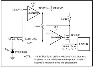
FIGURE 7. Precision Current Inverter/Current Source.
