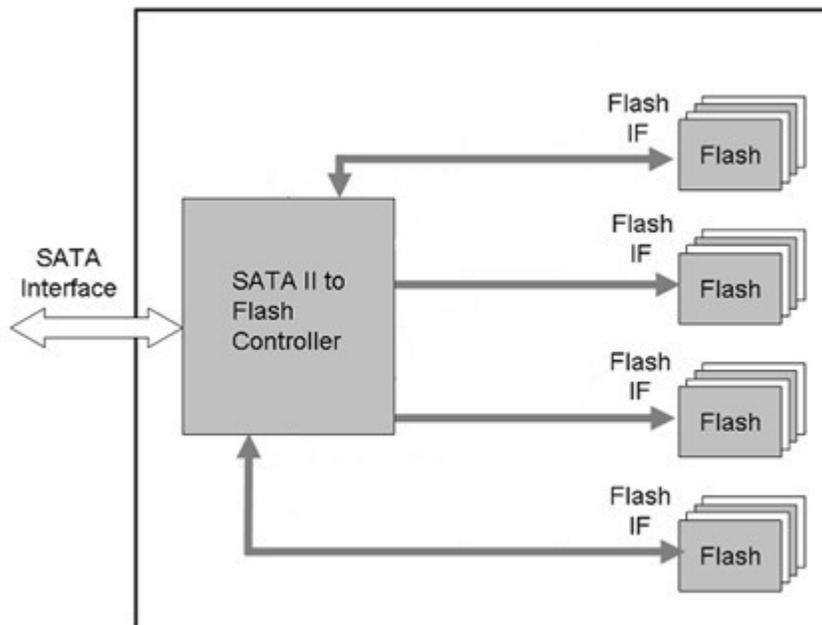
Figure 1-1 Apacer SDM II M1 block diagram
