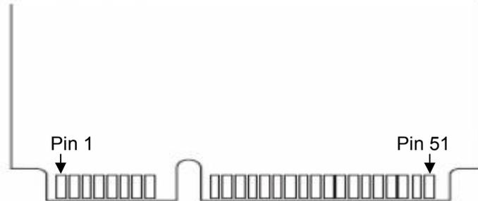
**Figure 1-2** Apacer SDM II M1 pin assignment
