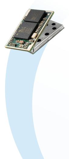
The BTM510 and BTM 511 are low-power Bluetooth<sup>®</sup> modules designed for adding robust audio and voice capabilities. Based on the market-leading Cambridge Silicon Radio BC05 chipset, these modules provide exceptionally low power consumption with outstanding range. Supporting the latest Bluetooth Version 2.1+EDR specification, these modules provide the important advantage of secure simple pairing that improves security and enhances easy use.
