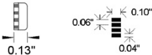
Figure 3: Suggested Pad Layout
