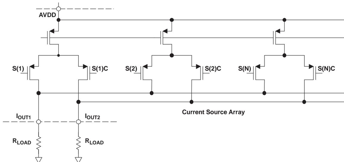
Figure 18. Analog Outputs
