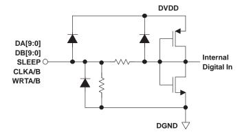
Figure 14. CMOS/TTL Digital Equivalent Input With Internal Pulldown Resistor
