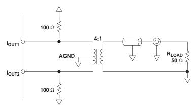
Figure 20. Driving a Doubly-Terminated 50- $\Omega$  Cable Using a 4:1 Impedance Ratio Transformer
