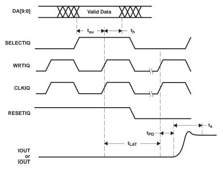
Figure 17. Single-Bus Interleaved-Mode Operation
