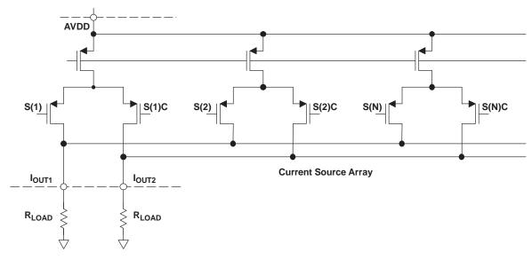
Figure 18. Analog Outputs
