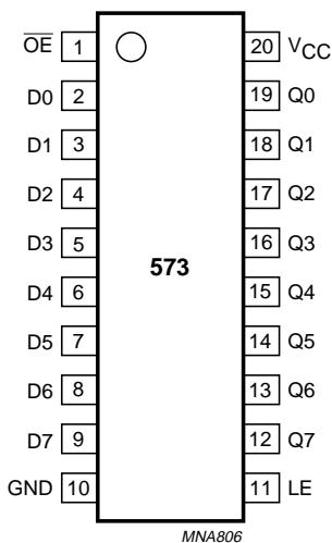
Fig.1 Pin configuration SO20 and (T)SSOP20.
