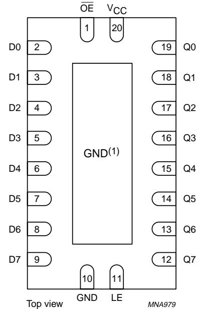
(1) The die substrate is attached to this pad using conductive die attach material. It can not be used as a supply pin or input.
