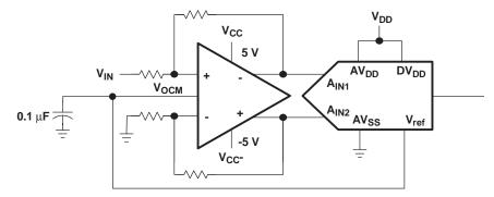
Figure 31. Fully Differential Amplifier Attached to a Differential ADC
