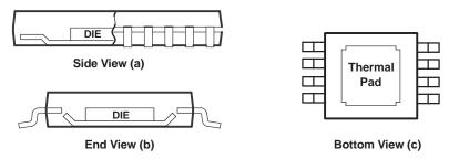
A. The thermal pad is electrically isolated from all terminals in the package.
