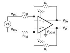
Note: For proper operation, maintain symmetry by setting  $R_f1=R_f2=R_f$  and  $R_{(g)}1=R_{(g)}2=R_{(g)}\Rightarrow A=R_f/R_{(g)}$
