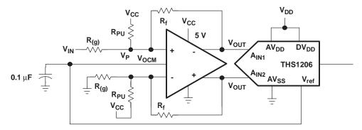
Figure 33. Circuit With Improved Common-Mode Input Voltage
