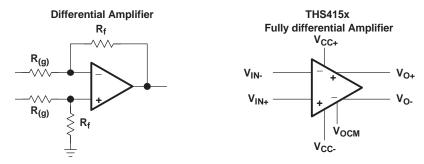
Figure 36. Differential Amplifier Versus a Fully Differential Amplifier
