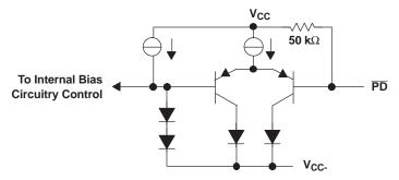
Figure 42. Simplified Power-Down Circuit
