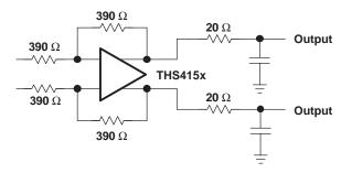
Figure 34. Driving a Capacitive Load
