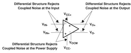
Figure 37. Definition of the Fully Differential Amplifier
