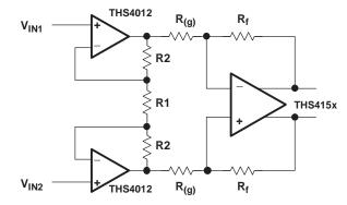
Figure 41. Fully Differential Instrumentation Amplifier
