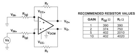
Figure 39. Single In With Differential Out
