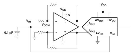
Figure 32. Fully Differential Amplifier Using a Single-Supply
