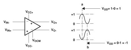
Figure 40. Fully Differential Amplifier With Two 1-Vpp Signals
