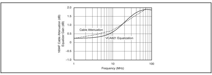
Figure 79. Cable Attenuation versus Equalizer Gain
