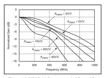
Figure 84. MSOP-10 Recommended  $R_{\text{F}}$  and  $R_{\text{G}}$  versus  $A_{\text{VMAX}}$
