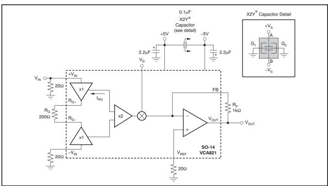
Figure 74. DC-Coupled, A<sub>VMAX</sub> = 20dB, Bipolar Supply Specification and Test Circuit
