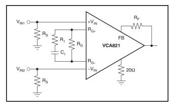
Figure 77. Differential Equalizer
