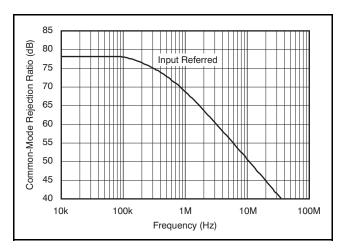
Figure 76. Common-Mode Rejection Ratio
