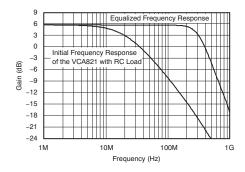
Differential Equalization of an RC Load
