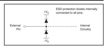
Figure 88. Internal ESD Protection
