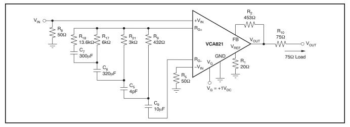
Figure 80. Differential Cable Equalizer
