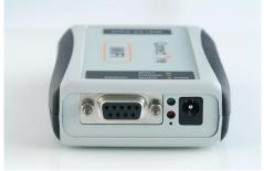
Side view: serial connector, power jack, mode select, SerialNET and power LEDs
