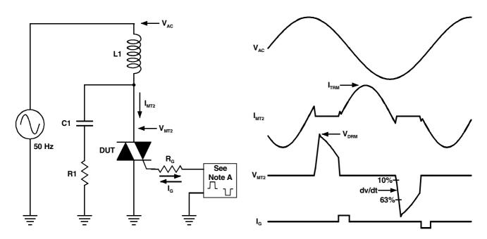
NOTE A: The gate-current pulse is furnished by a trigger circuit which presents essentially an open circuit between pulses. The pulse is timed so that the off-state-voltage duration is approximately 800 µs.
