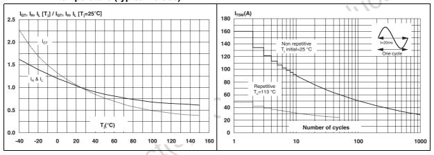
Figure 7. Non repetitive surge peak on-state current (sinusoidal pulse width tp<10 ms) and corresponding value of I<sup>2</sup>t
