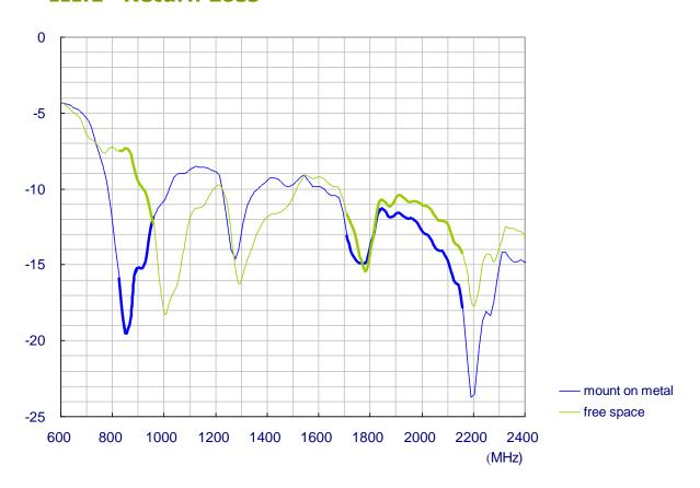
The highlighted parts are cellular operation frequency.
