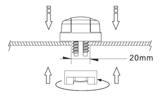
Recommended torque for mounting is 95Nm or 70ftlbs Maximum torque for mounting is 135.6Nm or 100ft lbs
