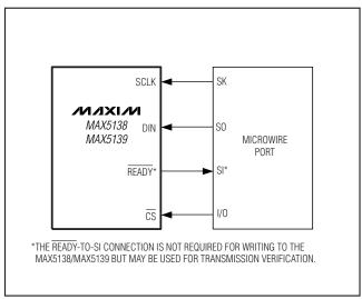
Figure 2. Connections for MICROWIRE
