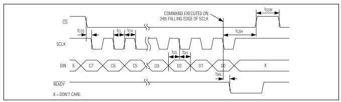
Figure 1. Serial-Interface Timing Diagram
