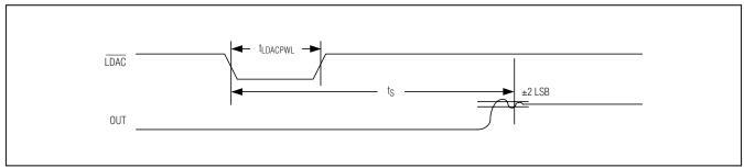
Figure 7. Output Timing
