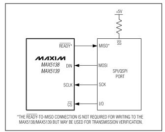
Figure 3. Connections for SPI/QSPI
